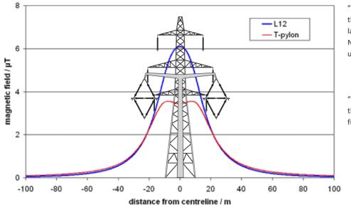
"L12" (in blue) is the standard steel lattice pylon that National Grid has used for some time.
